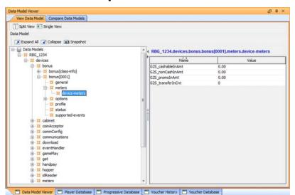
In addition to message responses, the **Data Model Viewer** lets you see the current data model. Using a tree-structure control, you can quickly drill-down to the attribute(s) or information you want to view. As you test, you can take snapshots of the data model for easy comparison of any two snapshots.
